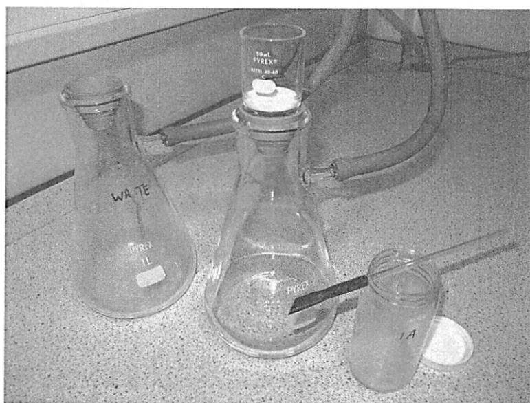
Fig. 2.4 Heavy-walled, 1 l Büchner flask with rubber ring adaptors; 250 ml Fisherbrand ® soda glass, wide mouth bottles with polyvinyl lined cap; and rubber policeman spatula.
